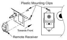
Figure 35 - Mounting Remote Receiver to Bracket
